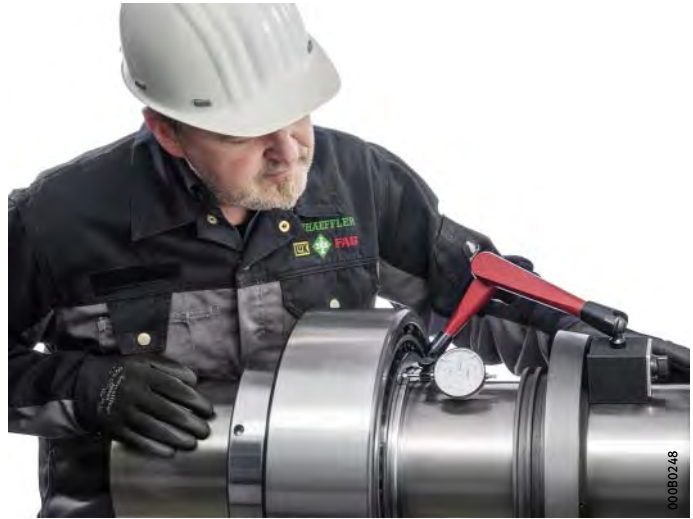
Figure 7 Mounting of toroidal roller bearing
