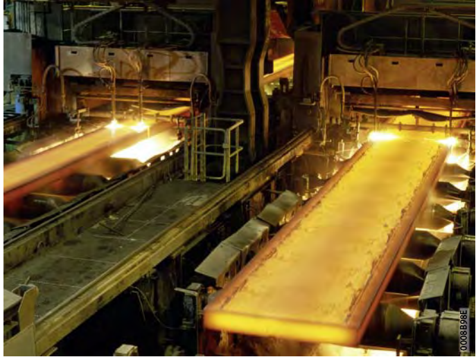
Figure 1 Continuous casting plant
